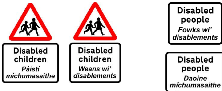
Bilingual “Disabled children” sign and “Disabled people” plate with Irish and Ulster-Scots (additional language at 80% size of English version)
