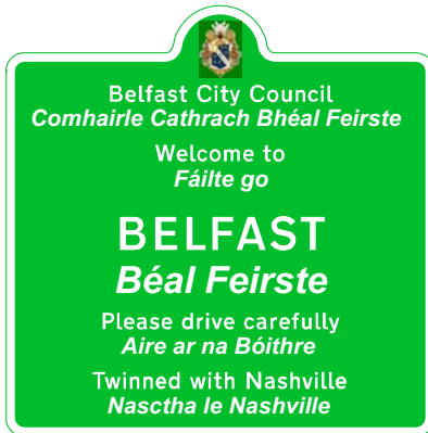
Figure 3 All sign elements replicated in Irish (2.7 x 2.7m 150 / 75mm x-height)
