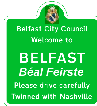
Figure 2 Bilingual version of place name only (additional language version of place name at 80% of English version) (1.9 x 2.1m 150 / 75mm x-height)
